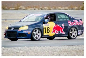
The Jetta TDI Cup car is powered by a 2.0-liter, 170 horsepower, four-cylinder TDI clean diesel engine mated to a six-speed, double-clutch, automatic DSG transmission
